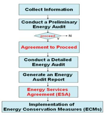
procedures, Determine the existing operating conditions of major energy use equipment (lighting, HVAC systems, motors, etc.), Estimate the occupancy, equipment, and lighting (energy use density and hours of operation)
